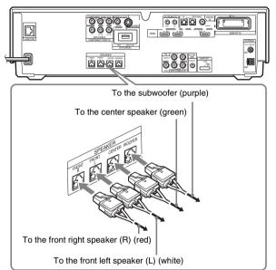
When connecting the speaker cords to the subwoofer, use the speaker cords (purple). Be sure to match the speaker cords to the appropriate terminals on the speakers: the speaker cord with the color tube to  $\bigoplus$ , and the speaker cord without the color tube to  $\bigoplus$ . Do not catch the speaker cord insulation in the speaker terminals.
